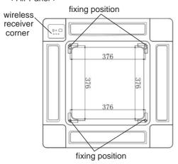
**Step 2**Mount the air panel onto the air panel fixing position by using the factory-supplied fixing screws (M5 screws).
