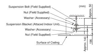
Fig. 4.7 Mounting Nuts and Washers
