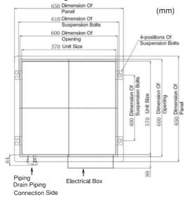
Fig. 4.3 Opening of False Ceiling and Suspension Bolts
