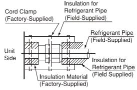
Fig. 5.3 Insulation on Pipes
