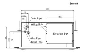
Fig. 4.6 Indoor Unit and Air Panel
