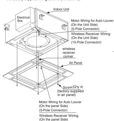
Fig.4.10 Installing Air Panel
