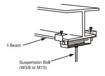
Fig. 4.4 Mounting the Suspension Bolts
