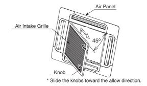
Fig. 4.9 Removing Method of Air Intake Grille
