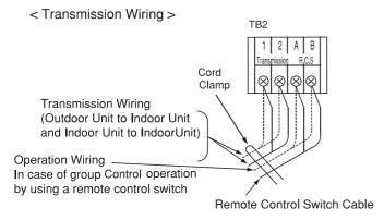
Fig. 7.2 Electrical Wiring Connection for Indoor Unit
